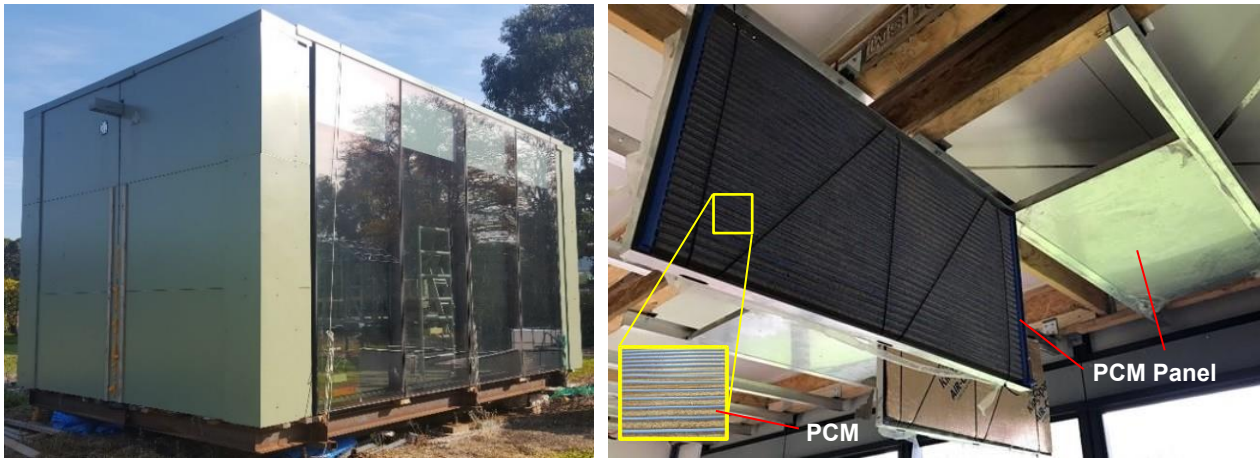
Fig. 4 The test cabin at the University of Melbourne (left), and PCM ceiling panels with capillary tubes (right)
