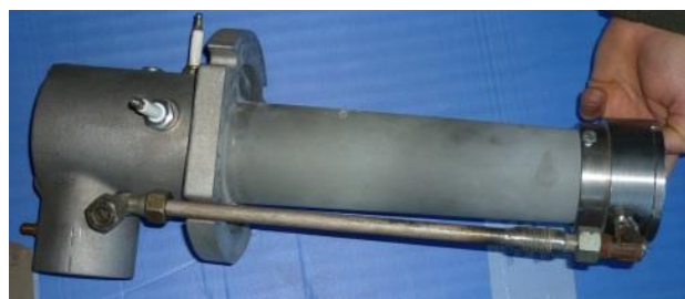
Fig. 2. Natural gas burner with attached annular sonic generator.
