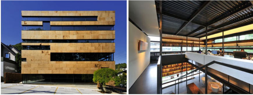
Fig. 16 The HIGO. Use of expanded cork cladding in building skin [41]
