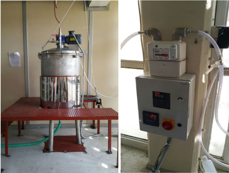
Fig. 2 Pilot-scale anaerobic digester (left) and control panel (right)
