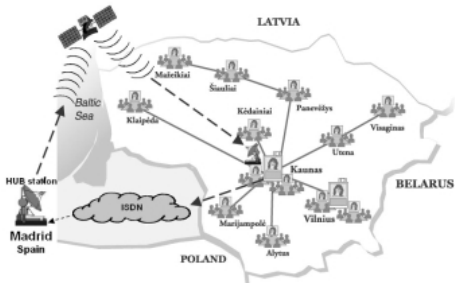
Figure 1: The integration of Lithuanian LieDM tele-learning videoconferencing network into Trans-European Tele-Education Network.
