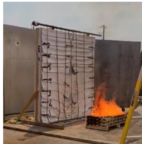
Example wall fire exposure.
