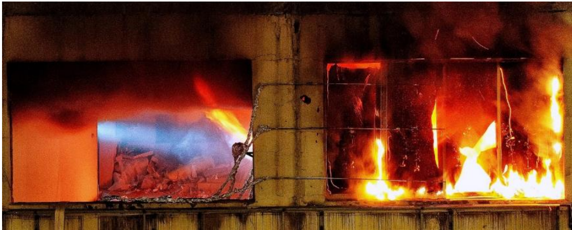
Burning urban village room and its ejected flame and smoke in an adjacent room
