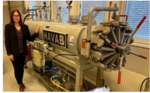
Edita near the industrial wood impregnation autoclave used to treat Scots pine sapwood.
