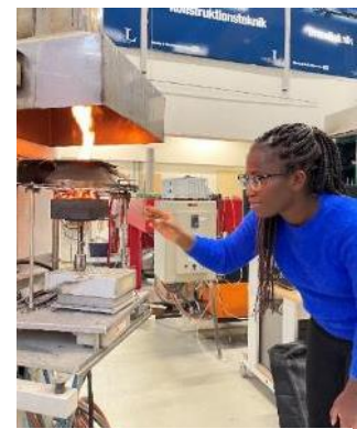
Rhoda performing cone calorimetry tests.
