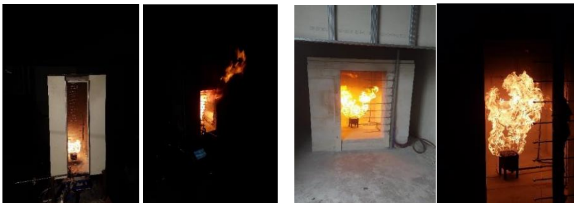
Setup of the small-scale experiments carried out at LEMTA (left) and the intermediate-scale experiments carried out at CSTB (right)
