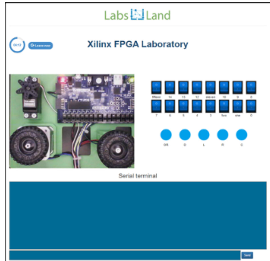
Figure 6. Debugging view of the WebLab-Deusto FPGA Remote Laboratory
