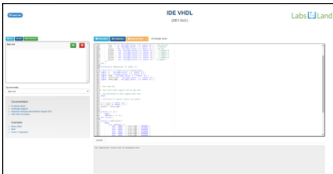
Figure 4. Interface of the WebLab-Deusto FPGA remote lab
