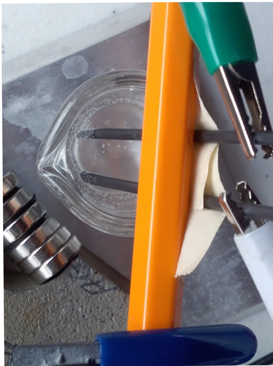
Figure 1. Sample experiment. Homemade magnetically-assisted solar water LED electrolysis.
